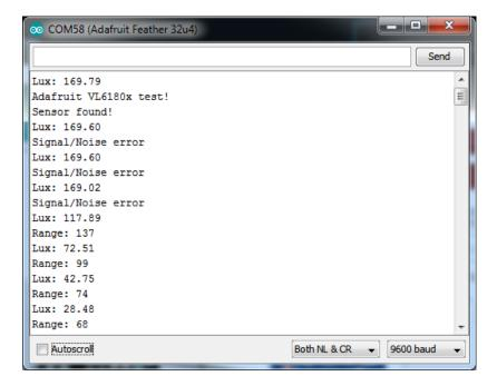
Move your hand up and down to read the sensor data, the range readings are in millimeters and the light sensors in Lux. Note that when nothing is detected, it will print out the error which may vary.
