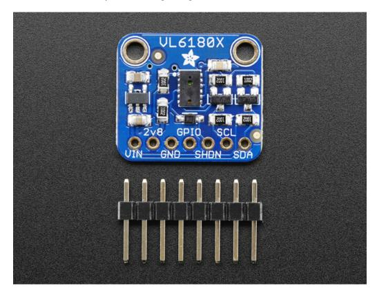
The sensor is small and easy to use in any robotics or interactive project. Since it needs 2.8V power and logic we put
