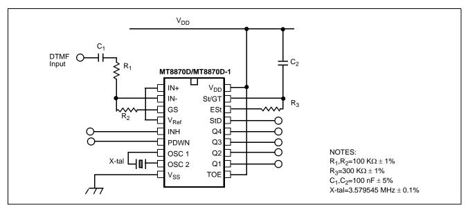
Figure 10 - Single-Ended Input Configuration
