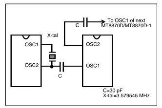
Figure 7 - Oscillator Connection
