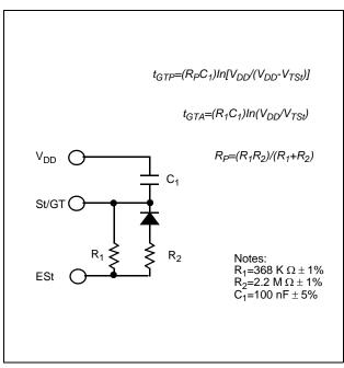
Figure 8 - Non-Symmetric Guard Time Circuit
