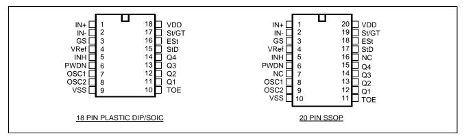
Figure 2 - Pin Connections
