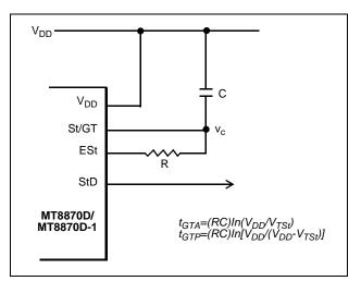
Figure 4 - Basic Steering Circuit
