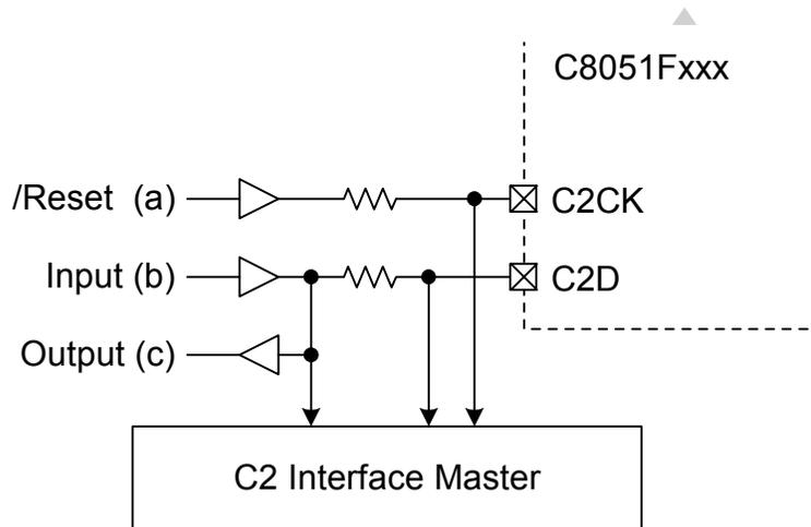
**Figure 26.1. Typical C2 Pin Sharing**
