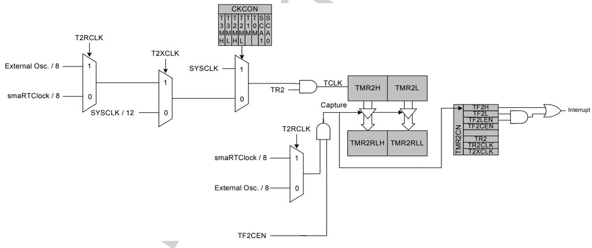
**Figure 24.6. Timer 2 Capture Mode Block Diagram**
