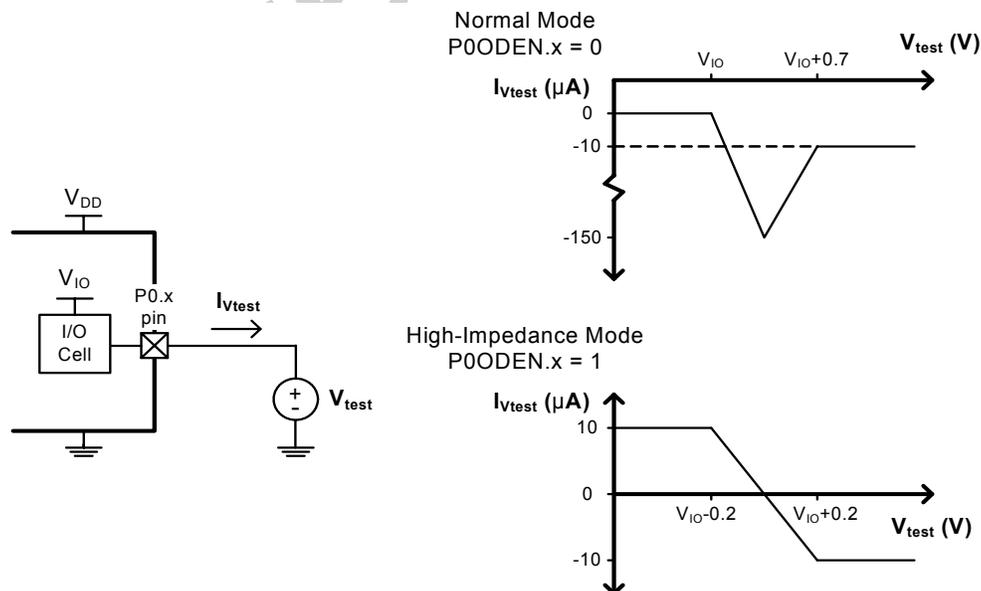
**Figure 18.5. Port 0 Input Overdrive Current Range**
