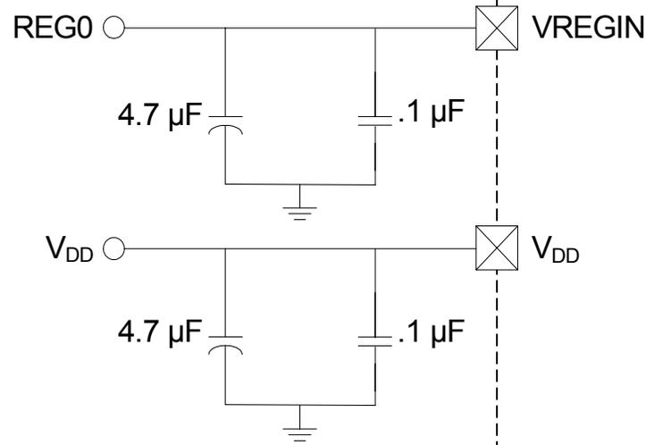
Figure 8.1. External Capacitors for Voltage Regulator Input/Output
