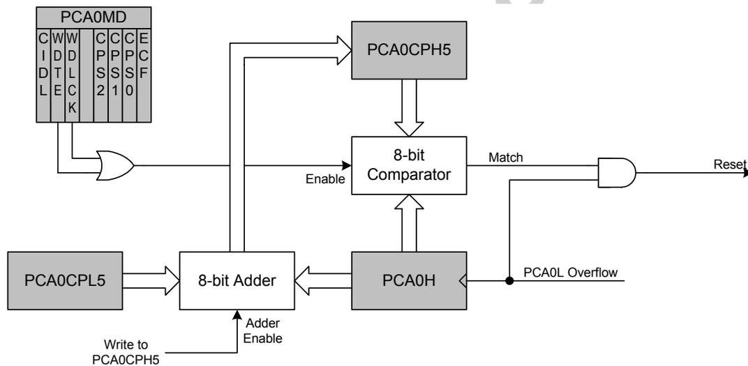
**Figure 25.10. PCA Module 5 with Watchdog Timer Enabled**
