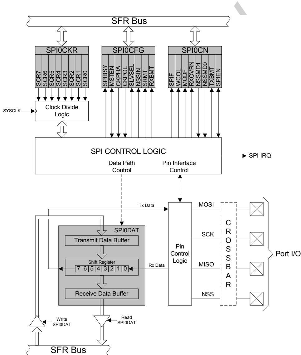
Figure 23.1. SPI Block Diagram
