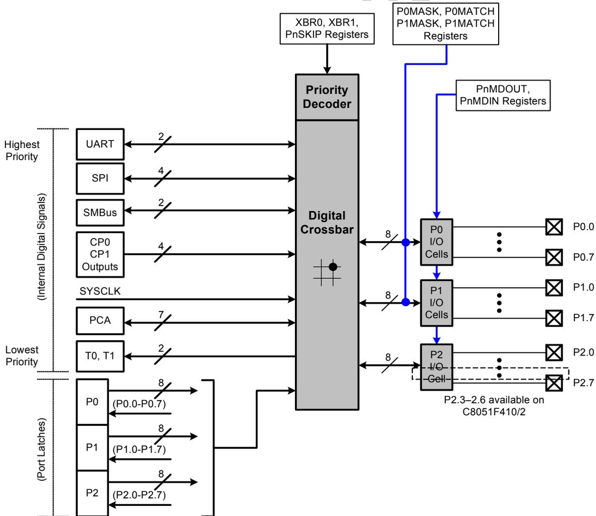
**Figure 1.11. Port I/O Functional Block Diagram**
