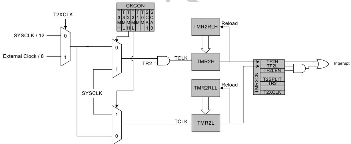
Figure 24.5. Timer 2 8-Bit Mode Block Diagram
