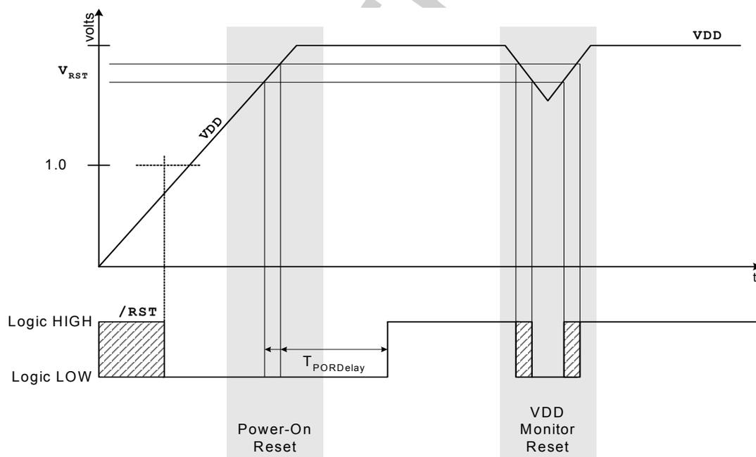
**Figure 15.2. Power-On and  $V_{\text{DD}}$  Monitor Reset Timing**
