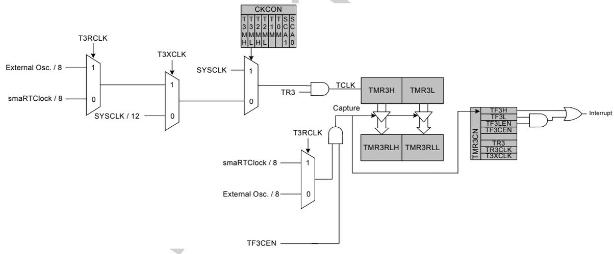
**Figure 24.9. Timer 3 Capture Mode Block Diagram**
