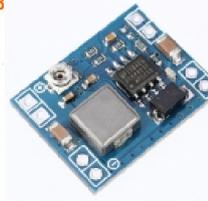
Mini DC-DC Converter Step Down Module Adjustable
