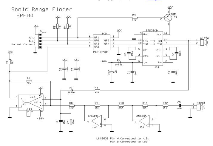
The circuit is designed to be low cost. It uses a PIC12C508 to perform the control functions and standard
